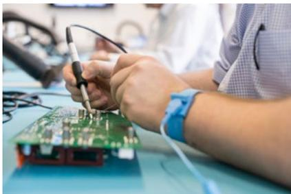
All Weller soldering stations are equipped with various options for potential equalization.
