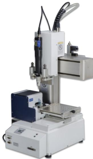
NSRI-B robotic device installation example
