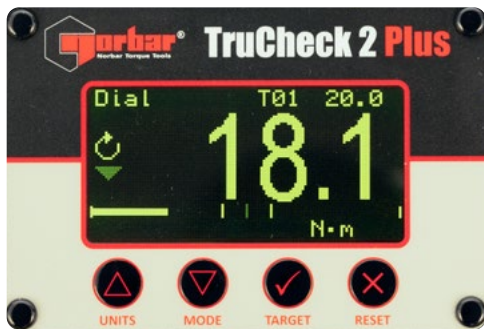
TruCheck™ 2 Plus display showing below target tolerance
