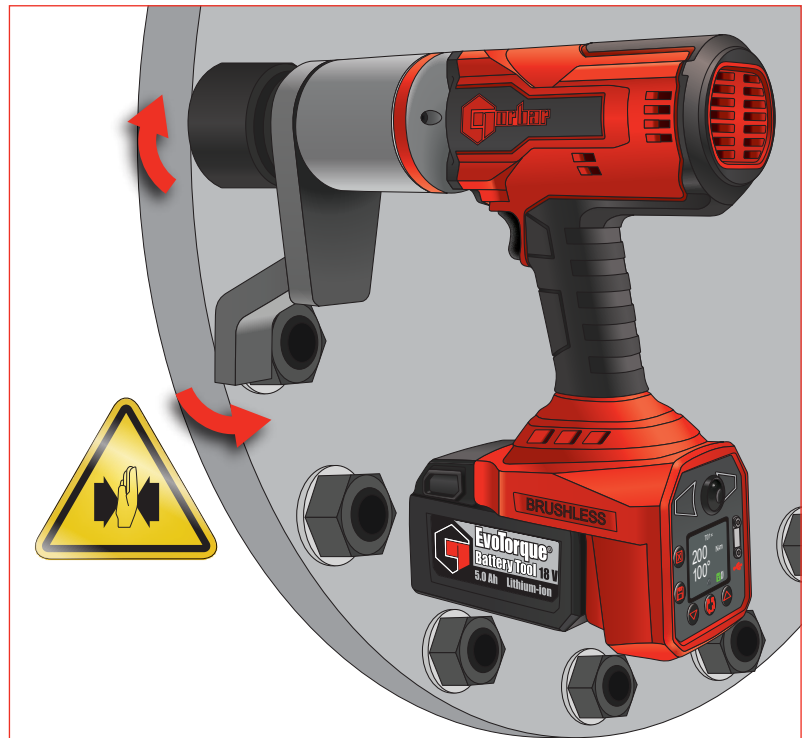
In the above example, 1,000 N·m torque output will result in a reactive force of 6,667 N at a point 0.15 m from the axis of rotation or 2,000 N at 0.5 m.
