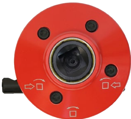
AWUR set to counter-clockwise operation
