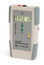
Large spectrum portable  $\Omega$  meter: from 0.01  $\Omega$  to 9, 99 10<sup>12</sup>  $\Omega$  (+/- 5%). Can test bracelets, floors, furniture, chairs and clothes by using electrodes (kit available separately).
