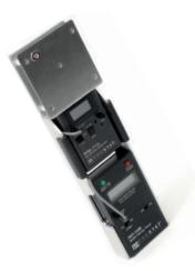
Allowing measurements of electrostatic field - discharge time. Ideal for calibrating and qualifying ionisers:
