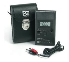
Voltage measuring: 0 to +/- 20,000 volt range, with increments of 1V and 10V
