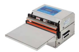
Nozzle type vacuum sealers are clean-room compatible and work well with all common vacuum bag materials. The unit uses a low noise, non-particle generating compressed air driven ejector vacuum pump which is efficient and maintenance free.
