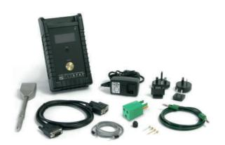
The New CVM-780 Contact Voltmeter combines the ease of use of a digital voltmeter with the high input impedance and low input capacitance of a true electrostatic voltmeter in a small, portable, battery operated package. Being a true electrostatic voltmeter, not a field meter means that it reads real voltage, without confusing it with electrostatic field strength, which can be distinctly different. Ceramic Probe Tips allow Accurate Measurement.
